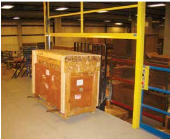
Vertical lift gate
